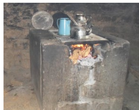
Figure 1 shows a deteriorated plancha stove in rural Guatemala. The stove is missing the chimney and the door at the front of the stove where wood is inserted into the fire. Large pots are cooked over the open fire (to the left) due to concerns that the metal stove surface will crack under the weight of the pot.
